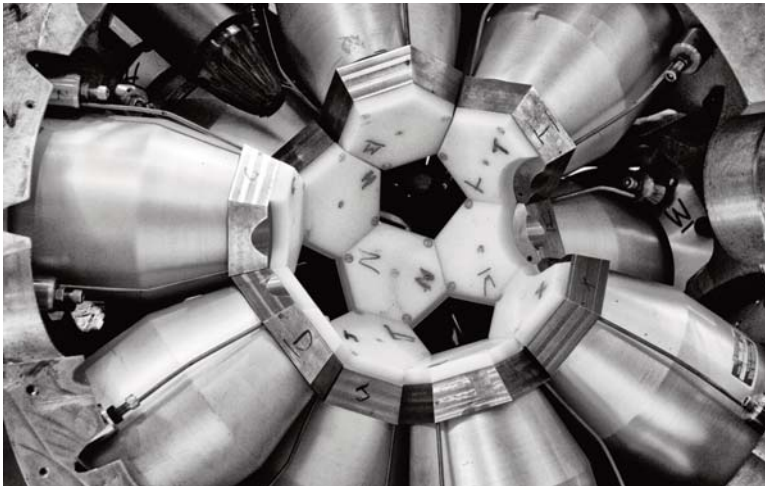
Figure 1: Photograph of the east hemisphere of the 8\pi spectrometer. Photo credit to Mikey Enriquez of the Global Photowalk 2010.
