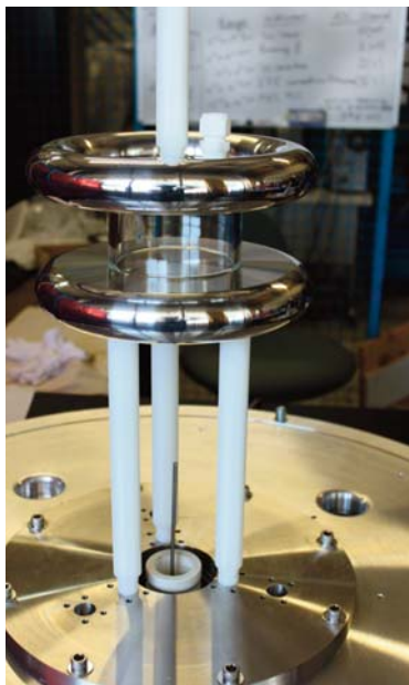
Figure 2: Left Top: Photo of Helium-II cryostat. The pumping for the He-3 and natural He (1 K) pots may be seen projecting out towards the viewer. Right: High voltage prototype of the storage cell for the measurement of the neutron electric dipole moment at TRIUMF. Left Bottom: Photo of cryostat. The long horizontal section that would connect the two cryostats is also shown.
