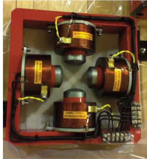
Figure 5: Newly designed and built short quadrupole for ARIEL, as it arrived in its packing crate, February 2013.
