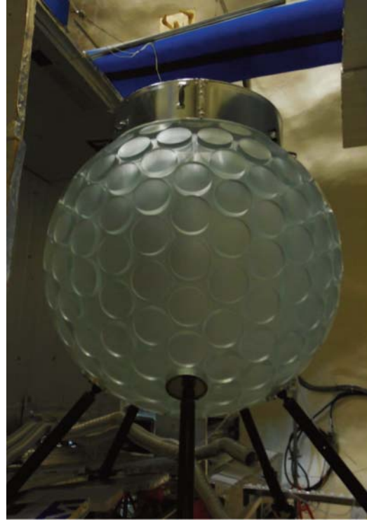
Figure 5: Acrylic vessel, underground at SNOLab.
