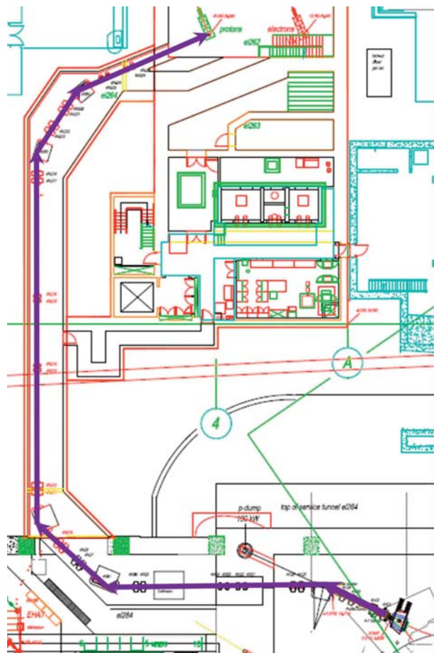
Figure 5: Phase 4 of completing ARIEL completes BL4N from the main cyclotron and carries protons to the west ARIEL isotope-production target.
