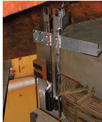
Figure 1: Neutral beam irradiation facility. The left-hand diagram shows a schematic of the NBIF, and the right-hand photo shows an ATLAS sample installed to the left of the NBIF ionization chamber.
