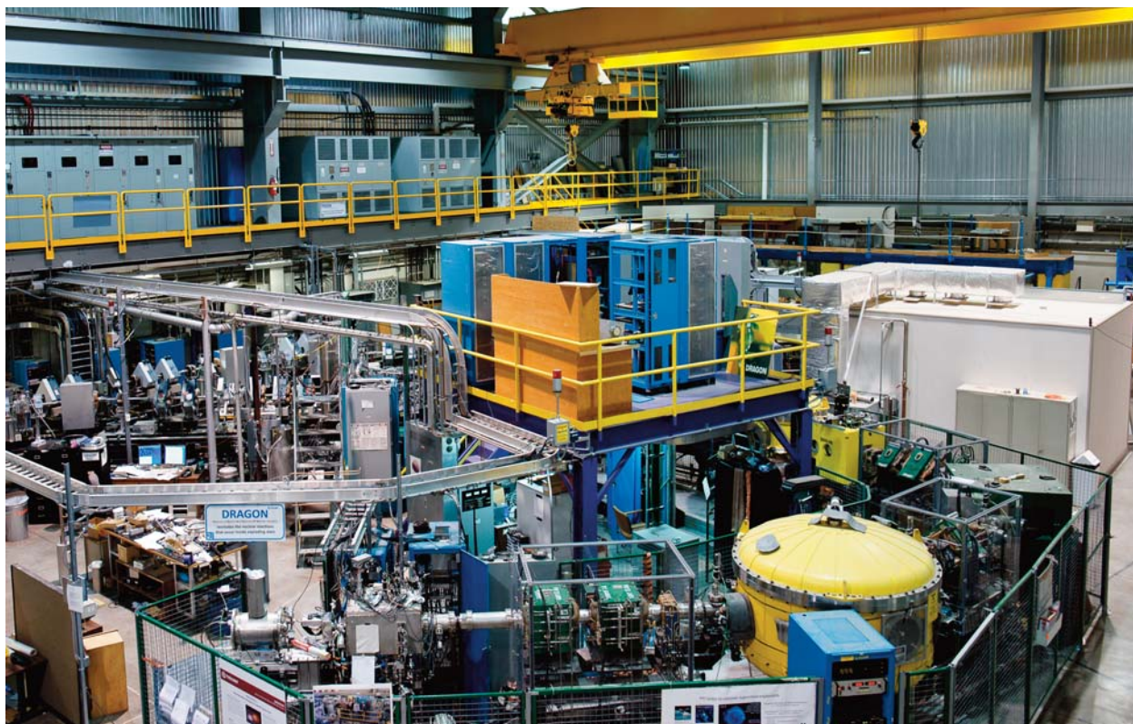
Figure 1: Plan view of the DRAGON recoil separator, showing the gas target where the nuclear reactions occur, the electromagnetic devices that separate the recoil nuclei from the unreacted beam, and the detectors that measure properties of the recoil nuclei. Photograph courtesy of Craig Damlo.
