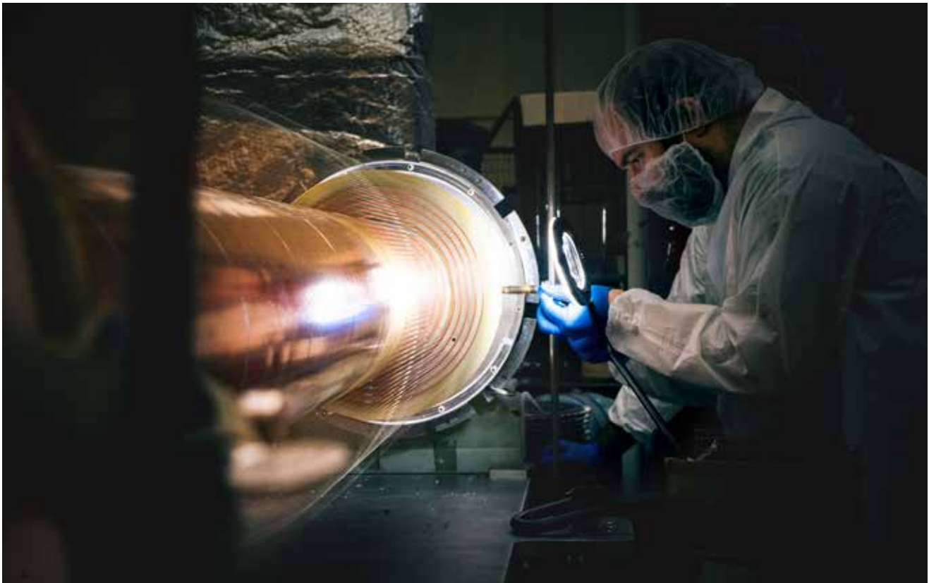
A TRIUMF physicist makes adjustments to the ALPHA-g antimatter detector, which was constructed at TRIUMF before being installed at the ALPHA experiment at CERN.
